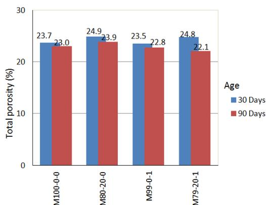
Figure 4. Total porosity of hardened mortars
