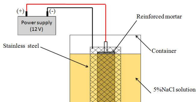
**Figure 1.** Experimental setup ACTIV assay.
