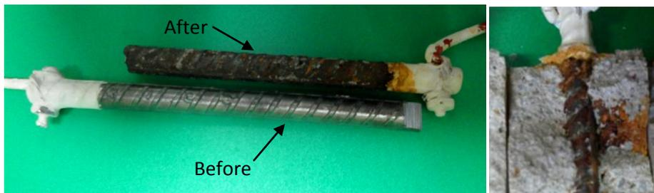
Figura 7. Reinforcing Steel after ACTIV.
