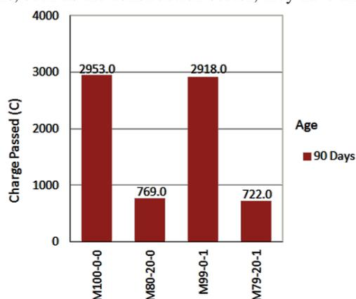
Figure 3. Total charge passed of hardened mortars according to RCPT
