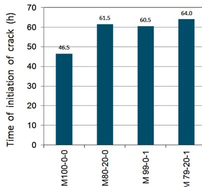
Figure 6. TIFC in assay of Accelerated corrosion test with impressed voltage.
