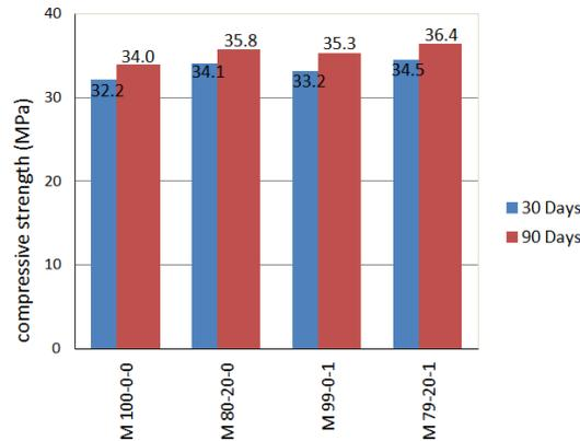
Figure 5. compressive strenght of hardened mortar.
